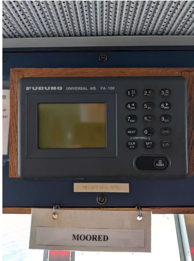
Figure 5. Installation Location for AIS
