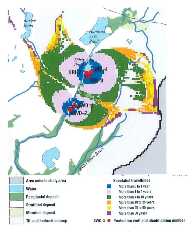
Figure 4 - USGS simulated groundwater travel times to production wells at their maximum pumping rates
