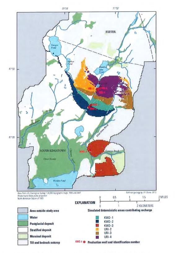
Figure 2-USGS Simulation of contributing recharge to the productions wells at maximum pumping rates.
