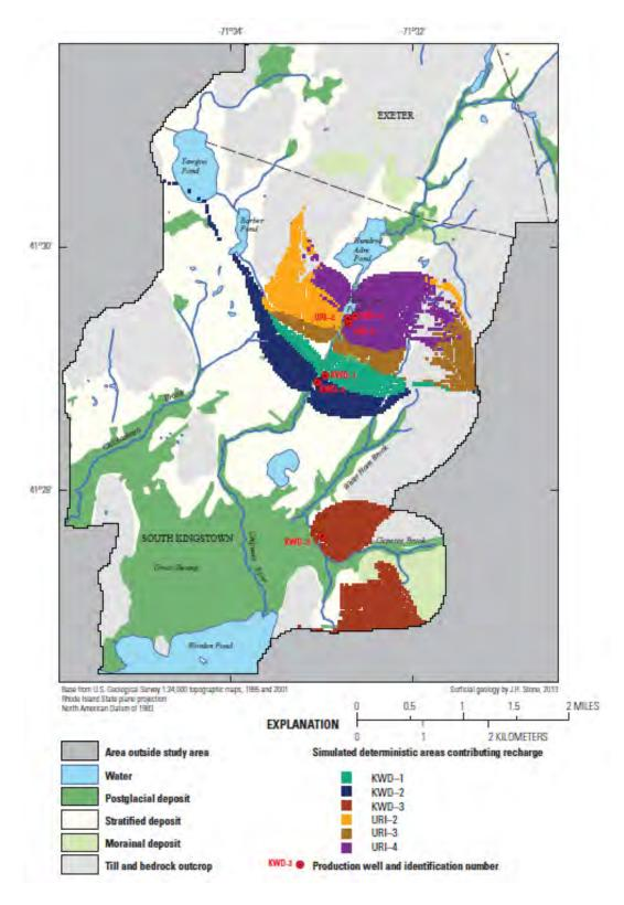
Figure 1- USGS Simulation of contributing recharge to the productions wells at maximum pumping rates.
